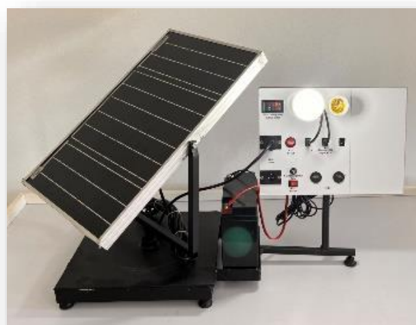
Figure 2 – Research stand for the physical characteristics of the photovoltaic panel
